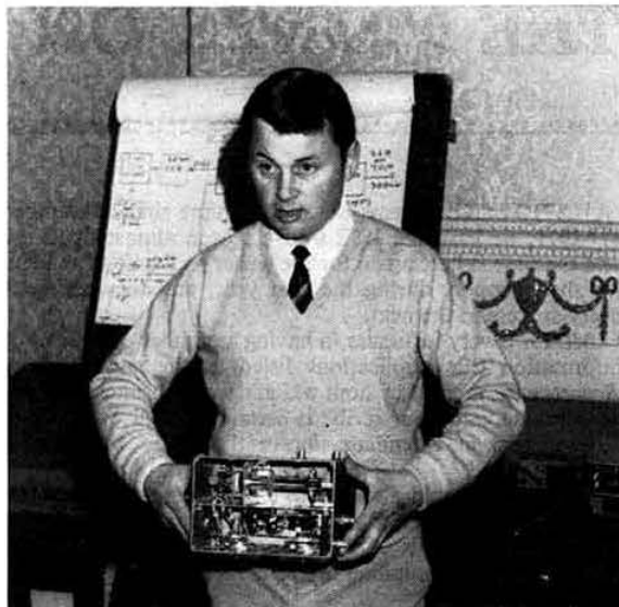
Arthur Russell, G8AWS, in action at a meeting of the Chester & DRS, when he demonstrated his solid-state 70cm sideband transmitter. Delivering 25W out, this rig will be behind GW8AWS/P on the Welsh hills throughout the winter whenever weather permits
